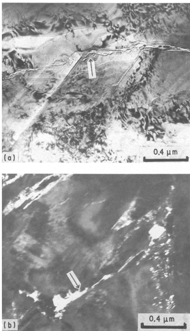
Figure 6 High-temperature substructures ( $T = 2500^{\circ}\text{C}$ ). (a) Crack in a diamond grain (indicated by arrow), (b) graphite segregations (dark-field image).
