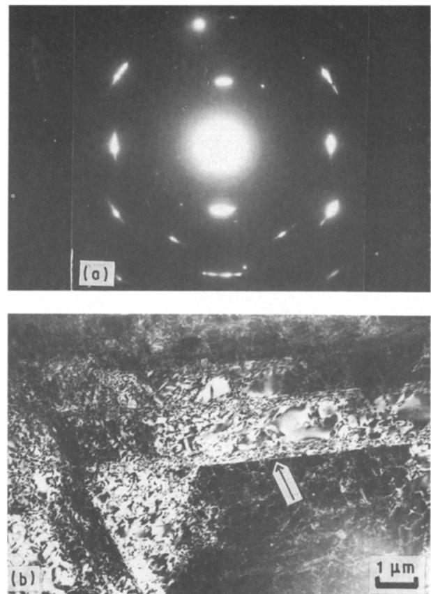
Figure 5 Fragmentation of grains. (a) SAD pattern from deformed region, (b) TEM image of deformed regions with disoriented boundaries (indicated by arrows).
