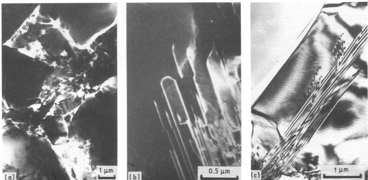
Figure 2 Details of substructure formed in the temperature range 700–1400 °C. (a) Submicrometre fraction of particles, (b) half-loops of perfect dislocations (dark-field image), (c) microtwins emitted from the particle surface.
