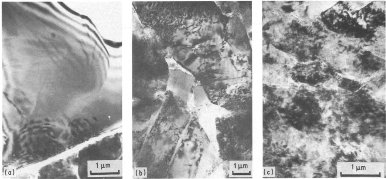
Figure 1 Transmission electron micrographs showing the defect density in diamond grains at different stages of  $P$ - $T$  treatment. (a) 700 °C, (b) 1300 °C, (c) 2100 °C.
