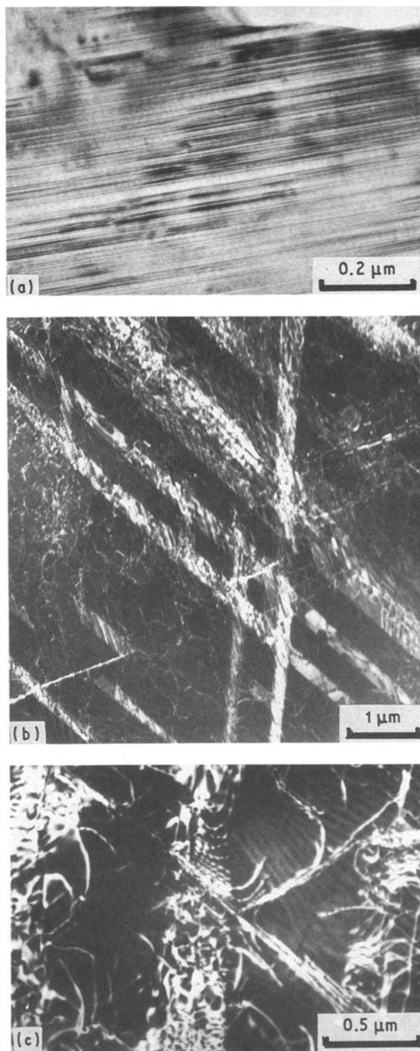
Figure 3 Microtwins in diamond grains. (a) The lamellar substructure, (b) intersecting microtwins, (c) dislocations on MT boundaries (dark-field images).
